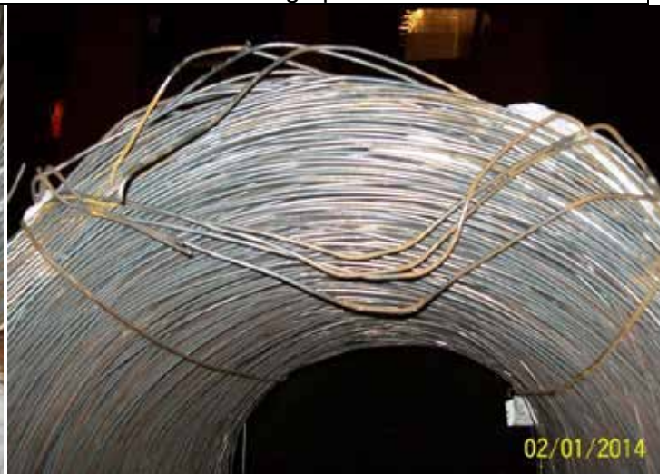
Damaged coils found
