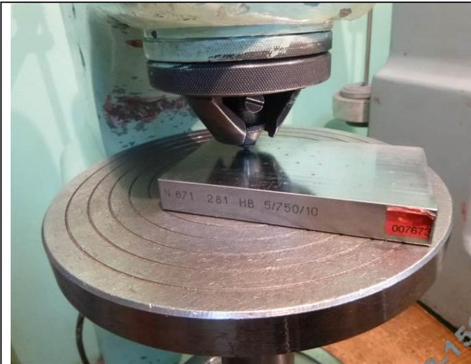
Photo 19 Hardness testing machine
