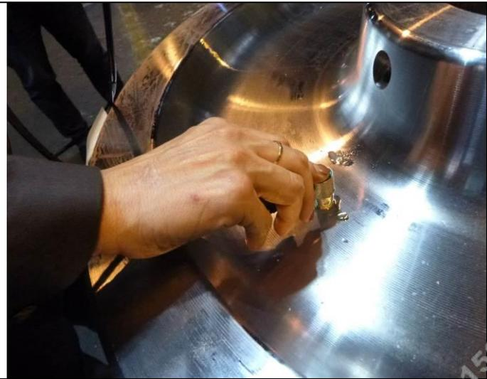
Photo 37 Web thickness measurement
